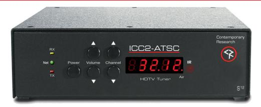
The ICC2-ATSC HDTV Tuner is an integrated HDTV tuner/controller that networks HD display monitors and projectors in an iC-Net and SignStream display control system. As a universal TV tuner, the ICC2-ATSC can receive ATSC, NTSC, and clear QAM cable channels from an MATV antenna or CATV cable RF system.
